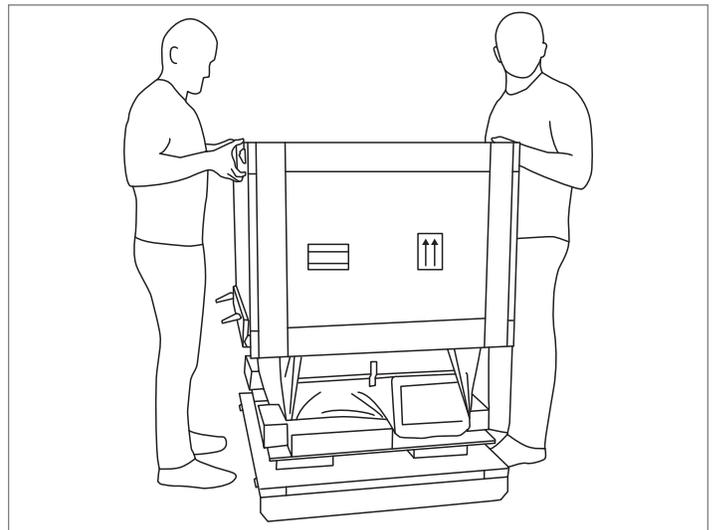
Figure 3: Placing the crate lid onto the base
